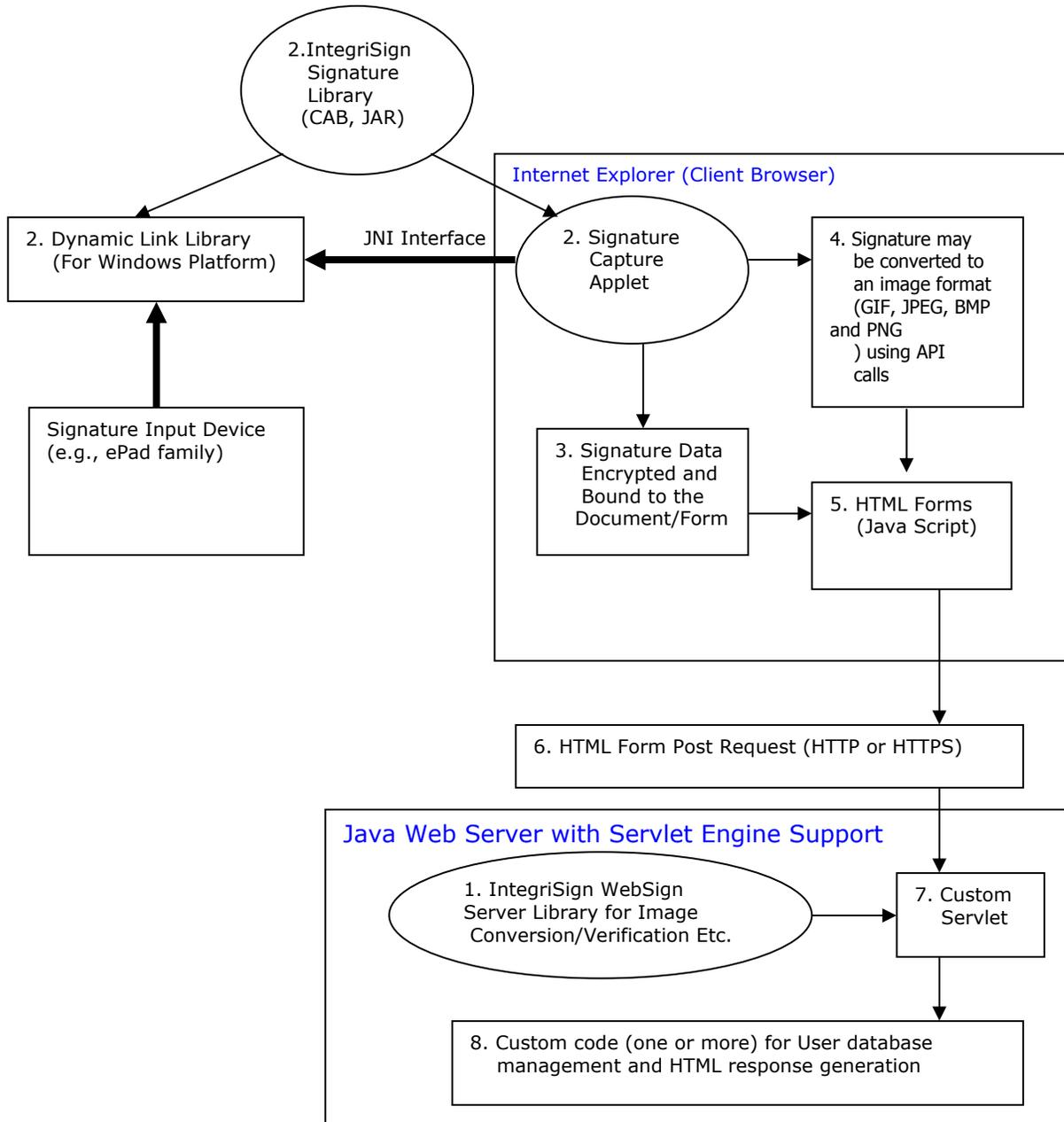
1. **Installation:** IntegriSign WebSign server Library along with the custom servlet is loaded onto the server. The downloadable distribution unit (CAB or JAR file) is also loaded onto the server and a reference is given to it from the HTML forms to be downloaded.
